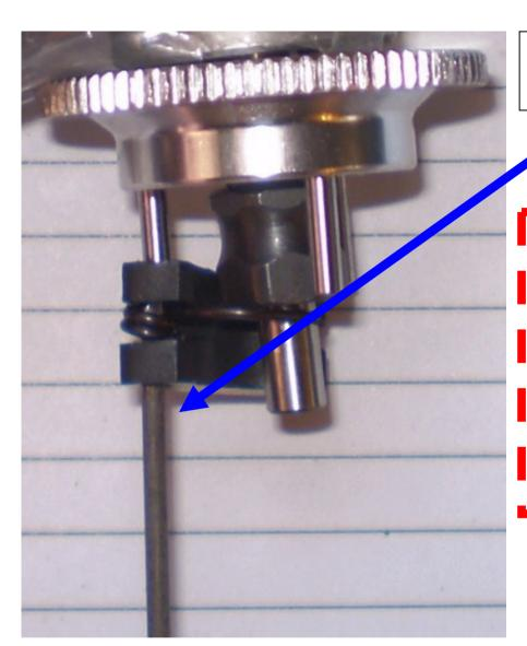
**Help — Clutch Assembly** The springs on the clutch shoes are very strong and difficult to assemble see photograph for the way in which we used a guide pin alternatively you can buy an Ansmann clutch installation too.
