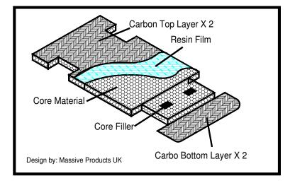
From the diagram you can see that this forms a simple composite laminated structure that can be cut roughly to shape prior to manufacture then cut and trimmed up later to exact size with simple hand or machine tools.
